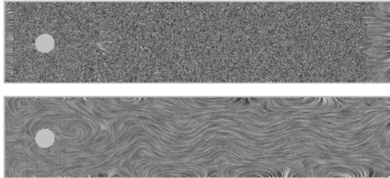
**Fig. 4.** Incompressible flow around a cylinder. Rotation-free component (top) vanishes except at inlet and outlet. Divergence-free component (bottom) has additional artifact at boundary. Courtesy Michael Hinze, TU-Berlin.
